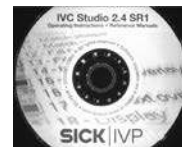
With ring light, more contrast, note the glare on the glossy center surface of the disc.
