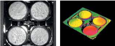
Even very slight height differences will be shown with 3D vision (right picture), the variation is hardly noticeable using 2D (left picture).
