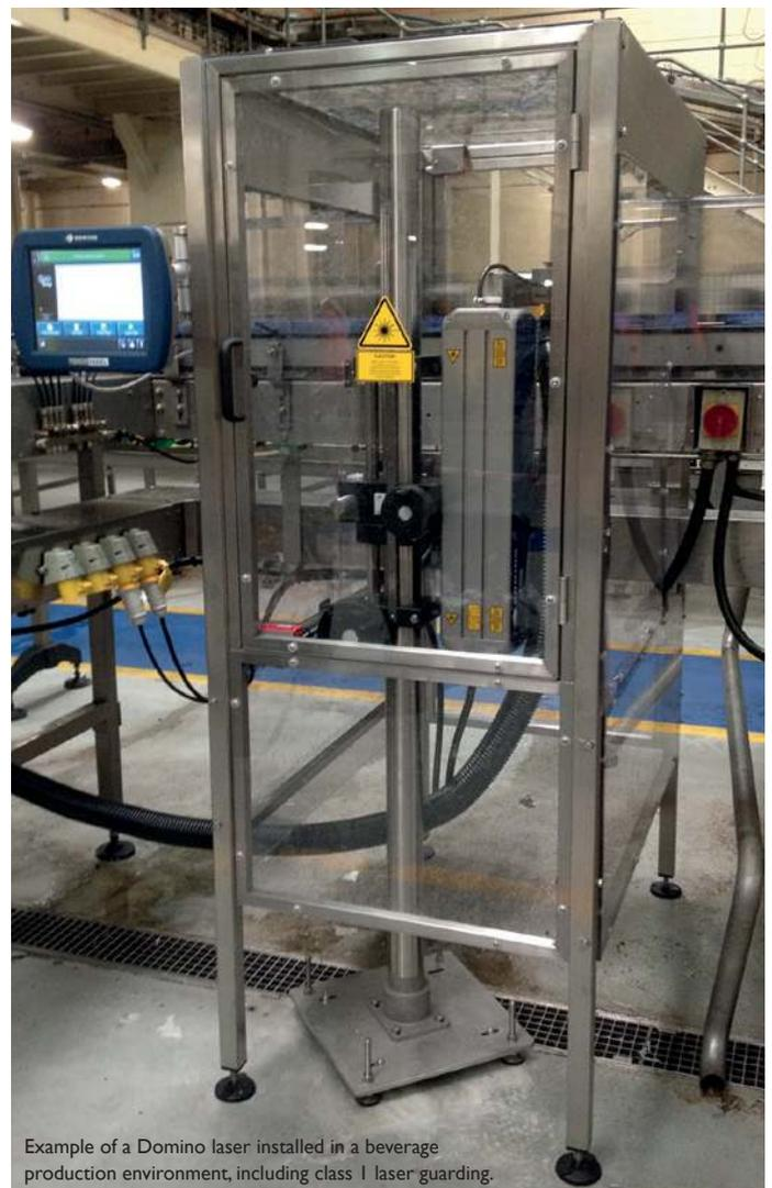
Example of a Domino laser installed in a beverage production environment, including class I laser guarding.
