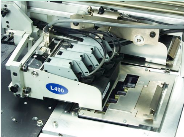
Bulk Ink print head entering M-Station
